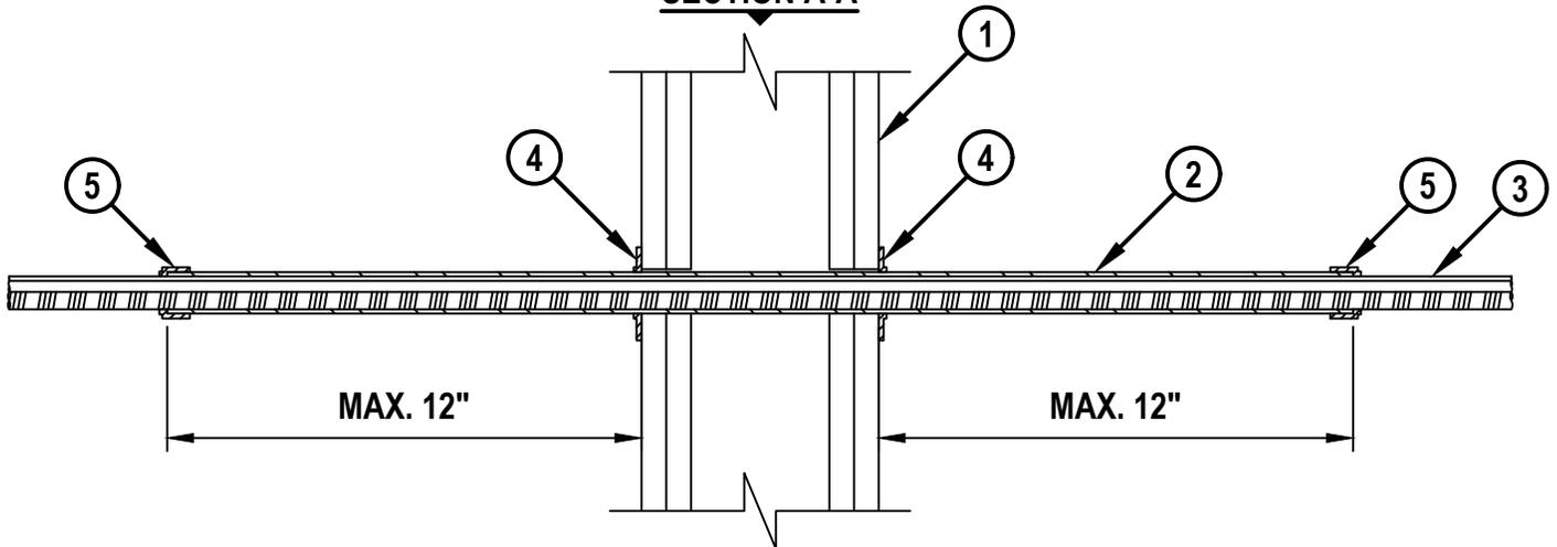
1. GYPSUM WALL ASSEMBLY (UL/cUL CLASSIFIED U300, U400, V400, OR W400 SERIES) (1-HR. OR 2-HR. FIRE-RATING) (2-HR. SHOWN) TO INCLUDE THE FOLLOWING CONSTRUCTION FEATURES :
