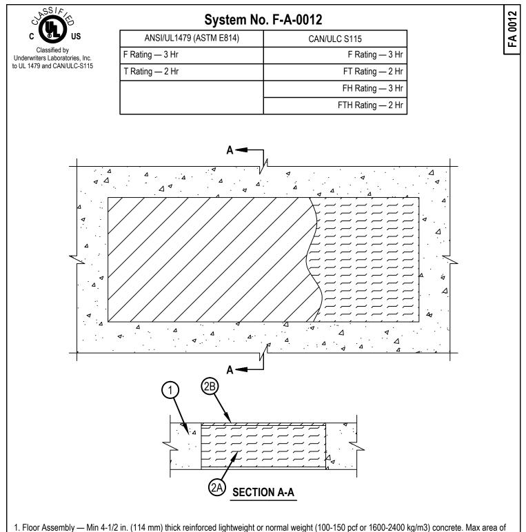
rectangular opening is 360 sq in. (2323 cm2) with max dimension of 30 in. (762 mm) or max diameter of circular opening is 12 in. (305 mm). 2. Firestop System — The firestop system shall consist of the following:
