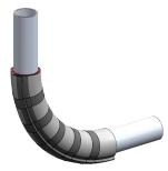
Prior to installing the adjacent straight sections, apply 1/8 in. wet thickness of CP 606 or FS One max over the entire edge of Hilti Endo-Shield Layer 1 (unless using collar protection).
