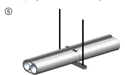
Apply 3 in. wide aluminum foil tape or FSK tape over the longitudinal seam.
