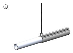
Wrap Hilti Endo-Shield tightly around the tubing overlapping 2 in. at the longitudinal seam. Apply 3 in. wide aluminum foil tape or FSK tape over the longitudinal seam.
