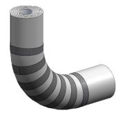
As per listing HI/AF 120-01. The elbow longitudinal seam of Layer 2 is located at the short radius of the elbow. The elbow longitudinal seam of Layer 3 is located at the middle radius of the elbow, rotated 90 degrees from the longitudinal seam of Layer 2. The elbow longitudinal seam for Layer 4 is located at the middle radius of the elbow, rotated 180 degrees from the longitudinal seal of Layer 3. The elbow longitudinal seam for Layer 5 (if necessary) is located at the long radius of the elbow.
