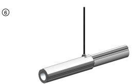
Wrap second layer of Hilti Endo-Shield in the same manner as Layer 1. The start of Layer 2 begins at the longitudinal seam of Layer 1, secured with 3 in. wide aluminum foil tape or FSK tape covering the full length of the seam. Radial seams can be treated in accordance with any of the seam methods outlined on the installation instructions for straight runs.
