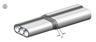
Offset the Layer 2 radial seam 2 in. from the radial seam of Layer 1. Tightly wrap Layer 2 over Layer 1 and overlap the longitudinal seam by 2 in. Cover the full length of the longitudinal and radial seam with 3 in. aluminum foil tape or FSK tape.
