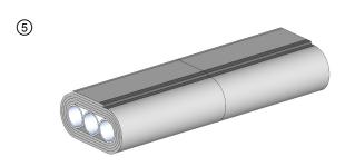
Apply 3 in. wide aluminum foil tape or FSK tape over the longitudinal seam.
