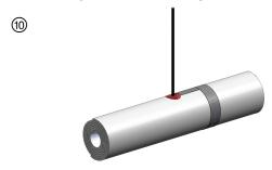
Apply 1/8 in. wet thickness Hilti CP 606 or FS-ONE MAX to outer diameter of the threaded rod penetration.
