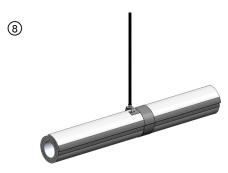
Apply 3 in. wide aluminum foil tape or FSK tape over the radial seam and overlap 2 in. onto itself. Add a piece of aluminum foil tape or FSK tape over relief cut.
