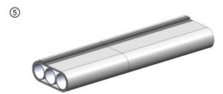
Apply 3 in. wide aluminum foil tape or FSK tape over the longitudinal seam.
