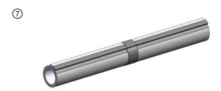
The radial seams are butted end to end without overlap. Apply 3 in. wide aluminum foil tape or FSK tape over the seam and overlap 2 in. back onto itself.
