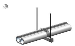
Apply 3 in. wide aluminum foil tape or FSK tape to wrap the strut ends.
