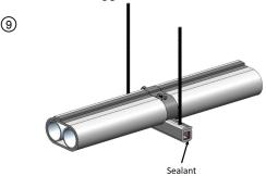
Apply 1/8 in. thick bead of Hilti CP 606 or FS-ONE MAX to the inner surface of the strut ends.
