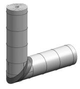
Tie an additional 3 pieces of min 18 Ga steel tie wire to existing wires, centered horizontally and vertically to form a basket around elbow protection.
