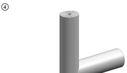
Install the adjacent continuously wrapped section. Both sections of Hilti Endo-Shield shall be slid together while aligning the 45 degree angled cuts.
