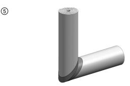
Apply 3 in. wide aluminum or FSK tape over the seam of the adjoining pieces of Hilti Endo-Shield.
