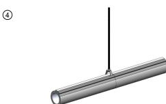
Traditionally critical conduits are supported with swivel loop hangers as shown in the picture above.
