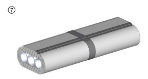
The radial seams are butted end to end without overlap. Apply 3 in. wide aluminum foil tape or FSK tape over the seam and overlap 2 in. onto itself.
