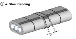
Secure collar with 1/2 in wide stainless-steel banding located 1 in. from each edge of collar as shown on the picture.
