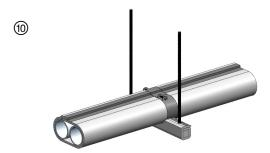
Cut a Hilti Endo-Shield plug to seal strut ends.
