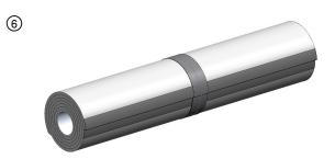
The radial seams are butted end to end without overlap. Apply 3 in. wide aluminum foil tape or FSK tape over the seam and overlap 2 in. back onto itself.
