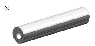
Apply 3 in. wide aluminum foil tape or FSK tape over the longitudinal seam.
