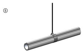
Apply 3 in. wide aluminum foil tape or FSK tape over the radial seam and overlap 2 in. onto itself. Add a piece of aluminum foil tape or FSK tape over relief cut.
