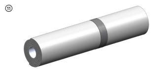
Layer 3, 4, 5: As required wrap third, fourth or fifth layer of Hilti Endo-Shield in the same manner as Layer 2 maintaining min 2 in. overlap of radial seams at each layer, to obtain desired rating.
