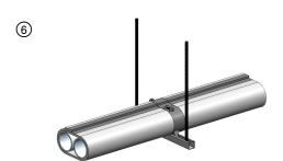
Apply 3 in. wide aluminum foil tape or FSK tape over the radial seam.
