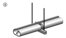
Prior to wrapping strut with Hilti Endo-Shield ensure additional 1/2 in. on both ends (this additional 1/2 in., that comes from the thickness of the product, creates a pocket for the Endo-Shield end plug) and include a 2 in. overlap on longitudinal seam. Apply 3 in. wide aluminum foil tape or FSK tape over the longitudinal seam.
