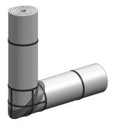
Tie an additional 3 pieces of min 1/2 wide steel banding to existing steel banding, centered horizontally and vertically to form a basket around elbow protection.
