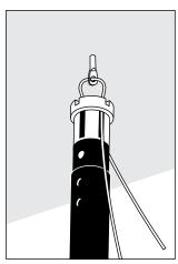
Lower the tool about 2" from base material surface as shown.
