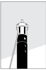
4. Raise tool against the ceiling, rotate the pole tool until the Eye Lag screw is at least 1-1/2" into the wood base material (embedment varies for steel base material CAUTION: In steel base material, stop turning before washer contacts base material to avoid stripping of the base steel.
