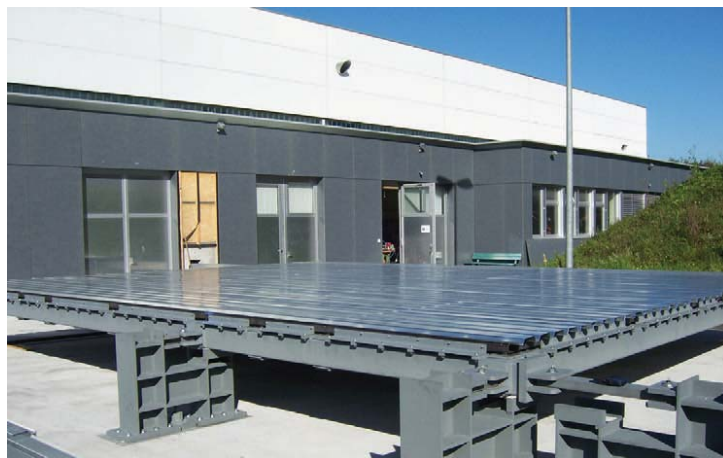
The test frame at the Fastening Systems Research Center in Schaan, Lichtenstein, simulates cyclic and seismic loading on an installed steel deck diaphragm.
