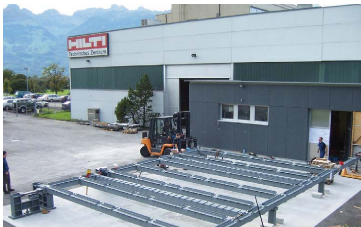
The test frame at the Fastening Systems Research Center in Schaan, Lichtenstein, simulates cyclic and seismic loading on an installed steel deck diaphragm.
